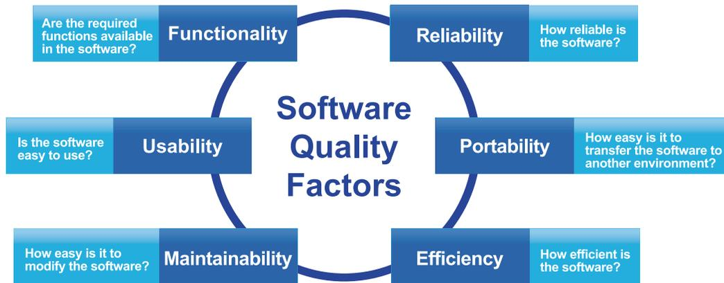
Figure 2: Software quality factors (source: [Agile Software Solutions](#))
